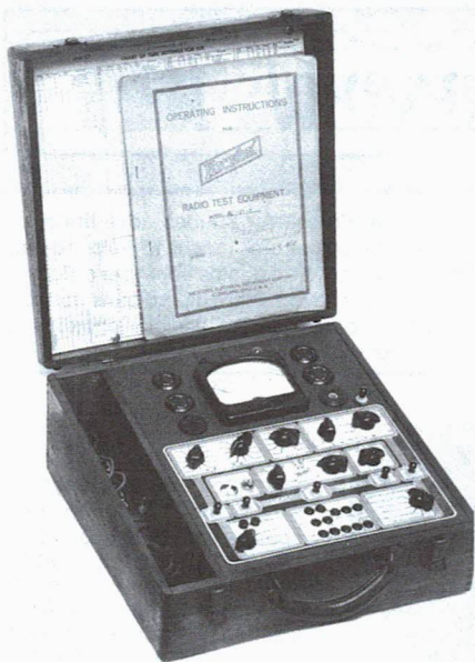
Figure 2. The Hickok Model AC51X tester is a combination VOM and tube tester.
