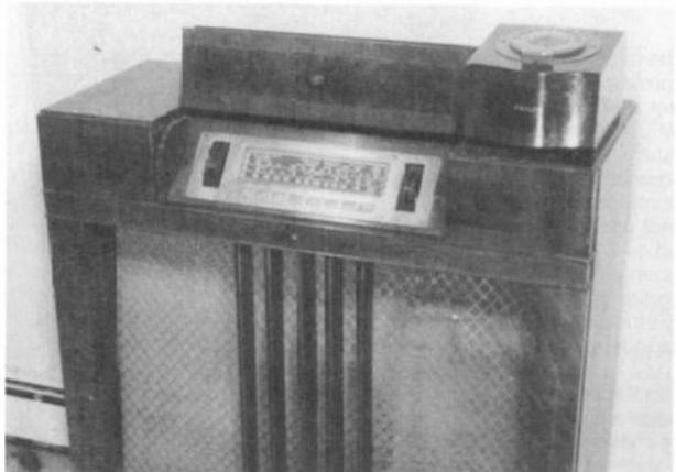
Figure 6. Philco introduced its wireless remote "mystery" control, shown atop a 39-116 console, in 1939.
