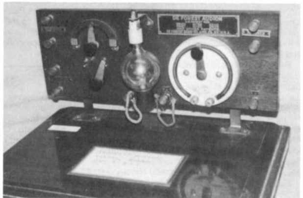
Figure 2. The De Forest RJ9 detector panel. (The non-original base and inventory tag were added for display purposes.)
