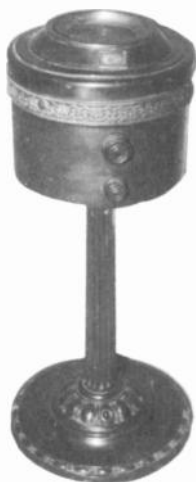
Figure 2. This General Motors preselector tuned stations, and used a remote radio as a fixed frequency receiver.
