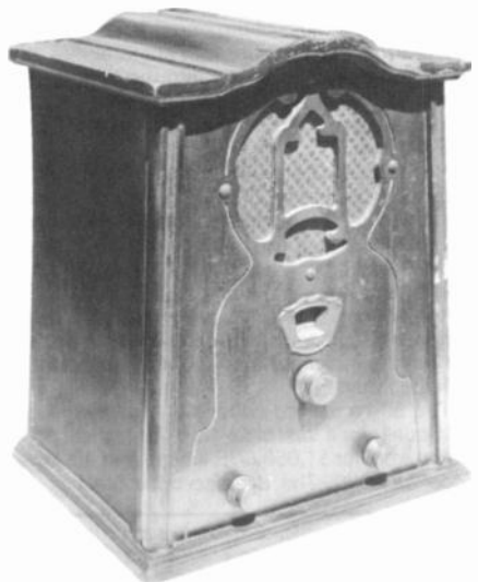
STEWART-WARNER MODEL R101-A – This cathedral radio, manufactured in the early 1930s, has an unusual shape. It is a basic 4-tube, AC broadcast receiver. The set is all original and even has the factory inspection tag on the line cord! (Robert Bailey – Jacksonville, FL)
