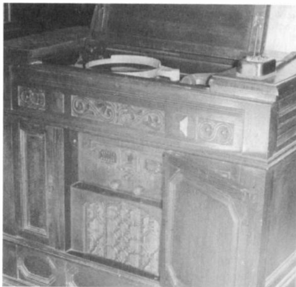
Figure 5. RCA's Model RAE-68 had motor driven automatic tuning with wired remote control.
