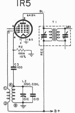
Figure 1. A partial schematic diagram showing a Type 1R5 used as a converter.
