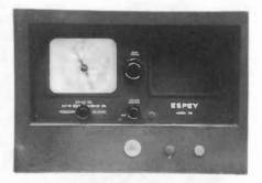
**ESPEY MODEL 581** – This 7-tube, .54 to 19 Mc receiver in a metal cabinet is similar in style to the Hallicrafters Model RE-1 Sky Courier, and also to the Minerva, which was on the August 1995 A.R.C. cover and in the April 1995 *Photo Review*. The cover holes are from previous modifications, for which the reasons are unknown. (Harry and Toni Blesy – Hinsdale, IL)
