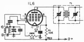
Figure 2. A partial achematic showing the use of Type 1L6.
