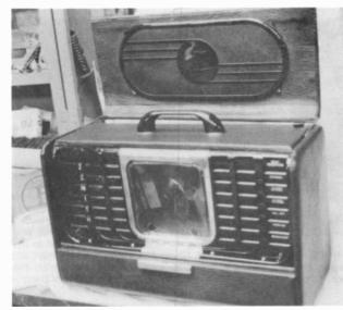
Figure 5. The restored Trans-Oceanic with its new covering and polished trim.
