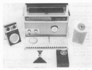
Figure 2. Representative American-made transistor radios shown clockwise from the top center: Zenith Royal 1000 Trans-Oceanic, Emerson 888. Regency TR-1, Philco T-7-126 and Zenith Royal 500.
