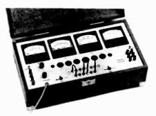
Figure 3. The author's tube-testing panel, constructed in a Western Electric oak case, using period Weston meters.
