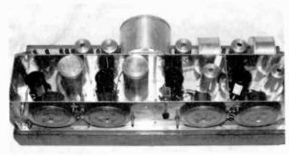
Figure 2. Top view of the radio showing the extensive shielding.
