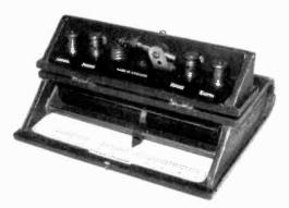
Figure 4. The leather-bound version of the Kenmac crystal set has an ivorine tuning scale.
