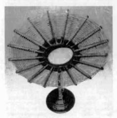
PARAMOUNT LOOP — This unusual loop antenna uses a Bakelite frame. It is about 15" tall and 12" in diameter, and all pieces are held together by wire. A tap bypasses about half the turns. The base is not original. (Richard Foster—Cochituate, MA)
