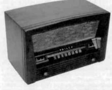
PHILCO MODEL 50-524 (522) – Although a typical 5-tube, AC/DC circuit, this model is unusual in that it uses three different tube styles including octals (2), loktals (2), and one 7-pin miniature. In 1950, Philco must have had an excess of loktals and octals and was phasing in the 7-pin miniatures. (Ralph Michelson – Brighton, MI)
