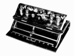
Figure 3. The tortoise-shell version of the Kenmac crystal set, shown with the cover open, features an engraved tuning-scale.
