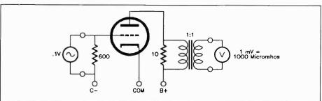
Figure 4. Basic circuit of the homemade tube tester. The actual instrument includes a high-pass filter to reduce hum pickup by the voltmeter.
