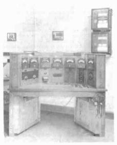
Figure 1. RCA's laboratory tube tester in 1928. The curves in the RCA tube manual were plotted using this sort of equipment.
