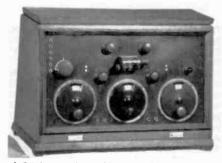
A 3-tube receiver with a panel-mounted crystal detector, this Mende E45, ca. 1926, sold for \$2,574.
