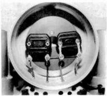
Figure 7. The output coupler and associated mica capacitors.
