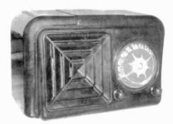
AUTOMATIC MODEL 614X - This 1946 AC/DC superhet was manufactured by the Automatic Radio Co., Boston, Mass., and uses the following tubes: Types 12SA7GT, 12SK7GT (2), 12SQ7GT, 35L6GT, and 35Z5GT. The cabinet is brown Bakelite and features a rather unusual "starburst" dial. (Douglas Fox - St. Charles, IL
