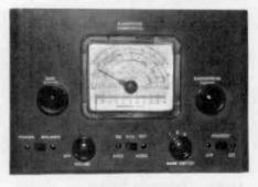
ECHOPHONE EC-1 - This Echophone Commercial was one of a line of very low cost communications receivers made by Hallicrafters. An early 1940s, little AC/DC set, it has 3 bands and BFO, and uses tube Types 12K8, 12SK7, 12SQ7, 12J5, 35L6, and 35Z5. (Doug Buskey - Mansfield, OH)
