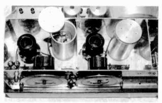
Figure 5. A view of the RF stages with shielded compartments, machined tube shields, coils, and variable capacitors.
