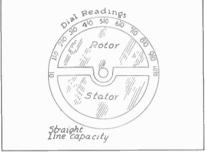
Figure 1. A straight-line capacity tuning condenser with its conventional semi-circular plates.
