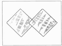
Figure 3. This unusual set of condenser plates will produce straight-line wavelength tuning.
