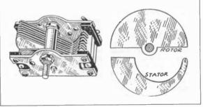
Figure 5. A version of a straight-line frequency tuning condenser that is much smaller than the unit shown in Figure 4. Note the semi-circular rotor and the odd shaped stator.
