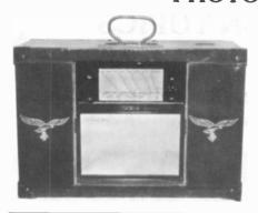
NORA RADIO TYPE K62 – This olive-drab colored, German-manufactured radio, found by a U.S. soldier in 1945, operates by battery or by a 220 VAC line. Depressing a button on top of the radio opens the two spring-loaded doors to reveal the control knobs, tuning dial, and speaker. The Nazi party emblem is displayed on the inside of the doors. A German officer's name appears on the speaker grille cloth. (Hank Trabold – Toms River, NJ)
