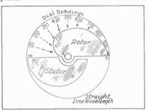
Figure 2. A straight-line wavelength tuning condenser with its shaped plates. Note the position of the rotor plates in relation to the dial reading.
