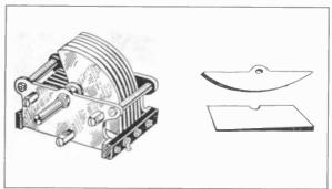
Figure 7. The use of plates that vary in thickness results in a compact straight-line frequency condenser.
