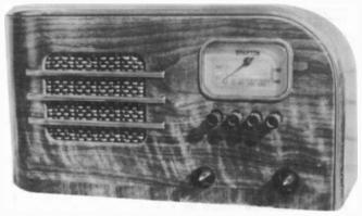
SPARTON MODEL UNKNOWN - This 5-tube radio is housed in a wood-grained metal cabinet with a chrome grille and trim. The tube types are 6A7, 75, 78, 42 and 80. (John Schehrer - Joplin, MO)
