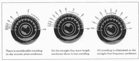
Figure 1. Examples of the relationship between tuning capacitor type and dial calibration.
