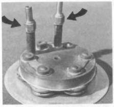
Figure 5. The entire diaphragm-button-cooling unit is removed. The arrows point to the water connections to the cooling chamber.
