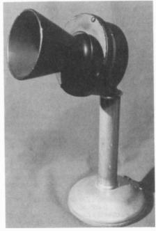
Figure 1. This example of one of Herrold's handmade, water-cooled microphones was mounted on a 1915 telephone base.
