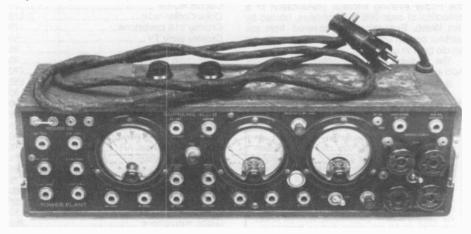
Figure 6. This Supreme Model 400B test oscillator and set analyzer uses an AC voltmeter, a DC voltmeter, and a DC ammeter.
