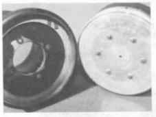
Figure 4. The mouthpiece is unscrewed to reveal a metal diaphragm bolted to the carbon "button" chambers.
