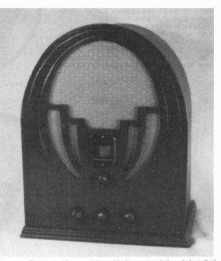
Figure 5. The finished new cabinet with the restored chassis installed and the escutcheon and knobs back in place.
