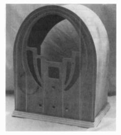
Figure 4. The cabinet completed with base trim cut on an angle from <sup>3</sup>/<sub>4</sub>-inch spruce.
