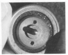
Figure 9. This close-up of the carbon button chambers reveals the granules inside.
