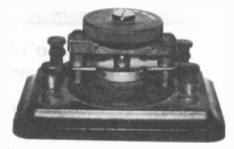
VETTER CARBON RHEOSTAT – This rare unit is 105 years old. The knob puts pressure on loose carbon contained in a cup. The carbon is held in place by a soft white rubber yoke, Only two binding posts are used. Two dummy posts balance the scientific Victorian era look. (Fred Geer – Jacksonville, FL)
