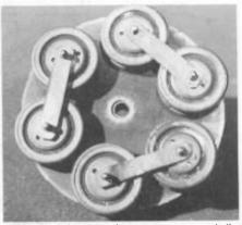
Figure 8. With the mica spacer removed, the series connections of buttons are revealed.
