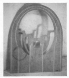
Figure 3. A front view of the new cabinet, showing the cutouts and the grooves cut in with an X-ACTO knife.
