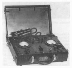
Figure 5. This Weston Model 566 Type 3 set analyzer accepts 4- and 5-pin tubes.
