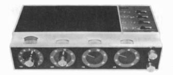
RCA MODEL UNKNOWN – This receiver for the visually impaired, circa 1970, features AM/FM, TV channels 2-13, and UHF reception. All controls have Braille markings, including the tuning drums protruding through a step-down front panel. (Fred Geer – Jacksonville, FL)
