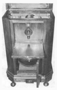
SPLITDORF "WARWICK" – This 1928 model has 7 tubes and is housed in a unique cabinet with a lid and drop-cover panel. (Steve Terlep – W. Melbourne, FL)
