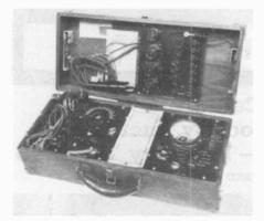
Figure 4. This Triplett test oscillator and set analyzer, mounted in a portable case, has test sockets for 4-, 5-, 6-, and 7-pin tubes and contains a multimeter.
