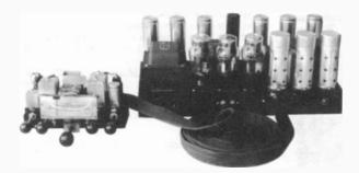
PACENT MODEL 9-R - This two-piece 1939 TRF set consists of an audio amplifier/power supply and a remote tuning head. The units are connected by a flat cable. The radio was designed for high fidelity broadcast reception in congested cities. It is the only radio made by this manufacturer of theatre equipment. (Clyde Watson -Scottsdale, AZ)
