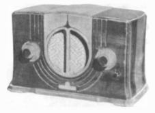
**GENERAL ELECTRIC MODEL L-53** – This AC/DC set is similar to an RCA Model 114. Five tubes are used — Types 78, 6A7, 77, 43, and 25Z5. (Joseph Loubriel – New Milford, NJ)
