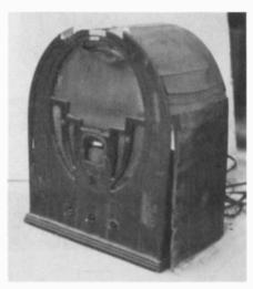
Figure 1. The sadly deteriorated Philco 60 as found, but with knobs and dial escutcheon removed.
