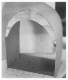
Figure 2. A rear view of the new cabinet under construction showing the arch support at top and the new plywood bottom.
