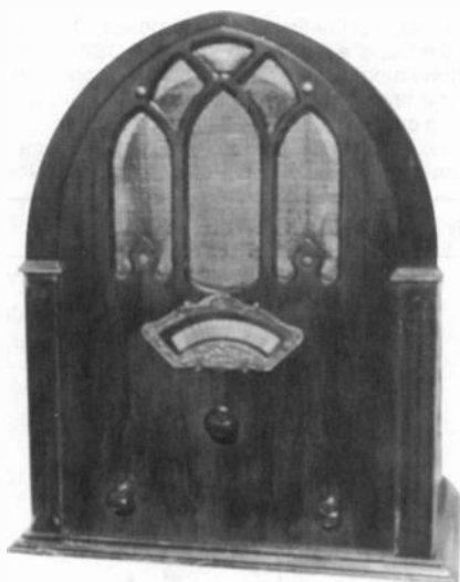
ARMRAD Type AC – This cathedral set is a very basic 5-tube TRF with Types 80, 47, 24, and (2) 35/51. It may have been made in New York, N. Y. Perhaps the name "Armrad" is a spinoff of Armstrong. ( Geoff and Wendy Shearer – Albuquerque, NM )
