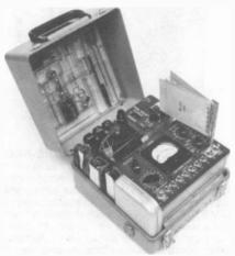
Figure 2. The USM-3A tool and tester kit, including the TV4 emission-type tube tester.
