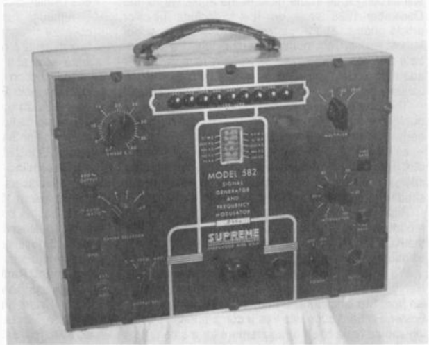
Figure 1. A Supreme Model 582 signal generator in a natural finish, tongue-and-groove wood cabinet with an etched front panel.
