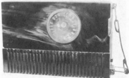
RCA MODEL 54B5 – This portable battery radio measures 6\frac{1}{8}'' \times 4\frac{3}{8}'' \times 3'' . It has a \frac{1}{4}'' -thick swirled plastic front and gold-finished metal sides. It uses a 1\frac{1}{2} -volt and a 67\frac{1}{2} -volt battery and has a built-in loop antenna. (Greg Farmer – Fridley, MN)
