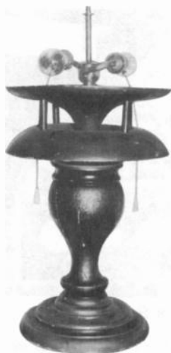
"THE ORACLE" – This unusual horn speaker/lamp was made by the Payne Co. in New York City. The driver is in the lamp base with the throat of the horn inside the lamp column. There is a sound diffuser near the top. "The Oracle" is embossed on the lamp finial, on a brass tag on the lamp, and on the speaker driver. (Greg Farmer – Fridley, MN)
