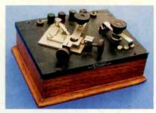
This Wireless Specialty Apparatus IP-175 silicon detector was one of the many crystal detectors offered. (Terrey photo)
