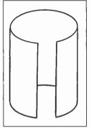
Figure 2. The cylindricalshaped paper diaphragm of the DeForest Audalion.
