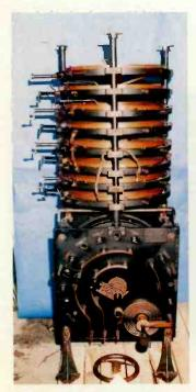
Washington Navy Yard oscillation-transformer assembly and wavechanger switch, one of the several 6' high, early spark transmitter components. (McElroy photo)
