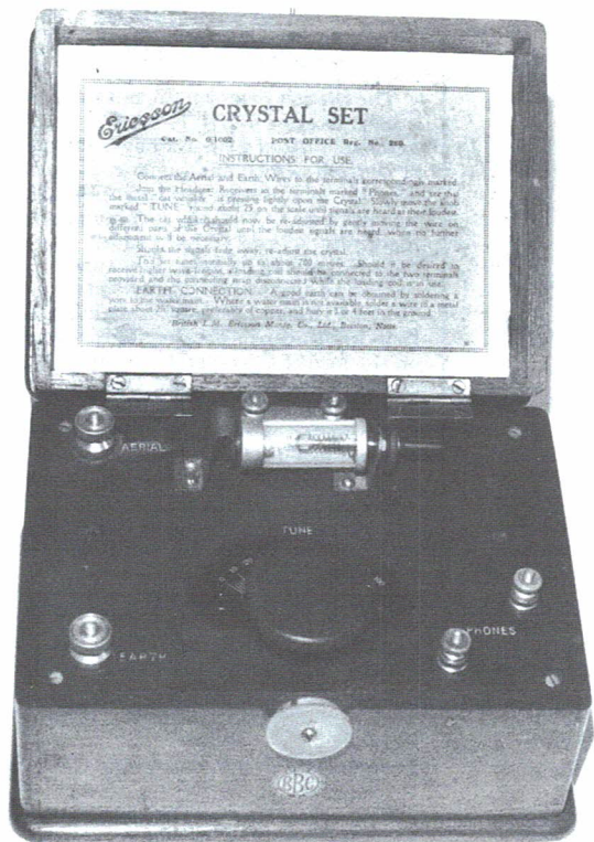
Figure 2. The later version of the Ericsson 0/1002 crystal set.
