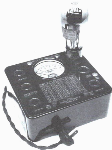
Figure 1. An early emission-type tube tester.
