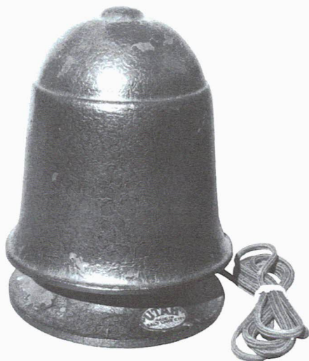
Figure 1. The Utah Super Flex horn speaker, which sold for $14 in 1925, is 8½ inches high and weighs 3 pounds.
