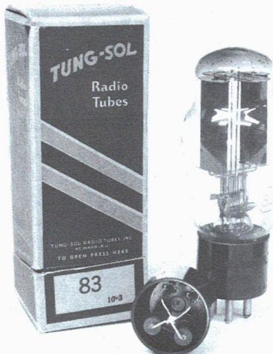
Figure 5. A Type 83 tube and its solid-state replacement.
