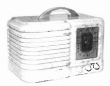
SENTINEL MODEL 212 – Listed in Rider's, Volume 12, page 1, this 6-tube Art Deco radio has a white plastic (Plaskon or urea?) cabinet with beautiful green and rust marbleing. It operates on shortwave frequencies of 5.7 to 18.3 MHz, as well as the broadcast band. Dimensions are 12" x 8" x 7". (Merrill Mabbs – Rapid City, SD)
