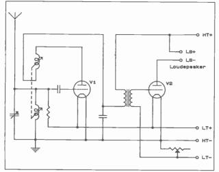
Figure 2. The circuit design of the Ethophone Duplex.
