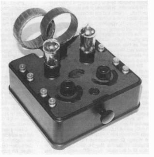
Figure 1. The Burndept Ethophone Duplex 2-valve receiver, shown here with two Mullard D.06 type valves.
