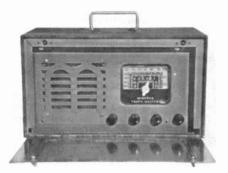
MINERVA TROPIC MASTER – This metal set was almost passed up at a flea market, as it looks like a power tool carrying case when closed! The set covers broadcast plus 5.5 to 19 MHz and has an RF stage and push-pull output (50L6's), which is somewhat unusual for an AC/DC set. Although it's not clear what market this set targeted, it looks as if it belongs to the Pan American flying boats era. (Tom Clinton [photo by Chuck Clinton] – Marietta, GA)
