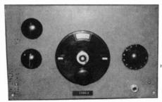
Figure 1. Front panel view of the 2-tube blooper built by the author in the late 1940s.
