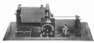
LOOSE COUPLER WIRELESS OUTFIT – This set was inspired by Arthur Harrison's article in the November 1992 A.R.C. entitled "Constructing Wireless-Era Receivers From Authentic Components." The unit uses an all-original loose coupler, a Tewno glass-enclosed tuning condenser, a Murdock loading coil, a phone condenser, and a DeForest crystal detector. (George Hausske – Wheaton, IL)
