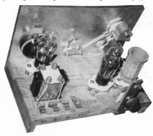
Figure 2. Interior view of the author's set showing the 2 Type 30 tubes.
