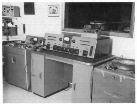
Figure 1. An RCA 76-B2 console (center), with an Ampex 300 tape deck (left), and a 16-inch transcription turntable (right).
