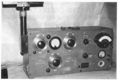
Figure 6. An RCA field strength meter with plug-in coil sets and loop antennas for four bands.
