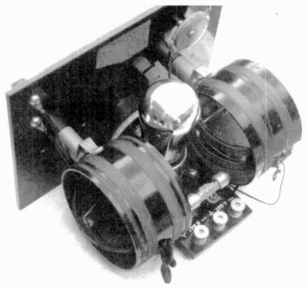
Figure 3. An interior view of the restored Echophone Model J, showing the simplicity of its design.
