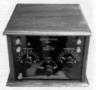
Figure 1. The restored Echophone Model J receiver.
