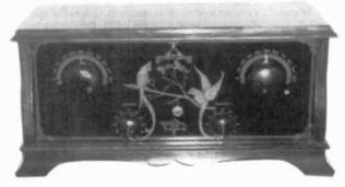
ROYAL RADIO CORP. POLLE **ROYAL MODEL** – Manufactured in Cranston, Rhode Island, this 1920s tube battery set is a great performer. The right tuning knob controls two ganged capacitors in RF stages, while the left one tunes the antenna circuit. (Herb Parsons - Peabody, MA)
