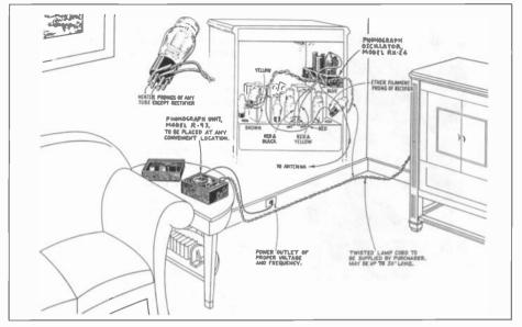
Figure 2. Typical installation of the RCA R-93 phonograph and the RK-24 phonograph oscillator.
