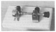
Figure 4. The Clapp-Eastham Universal Ferron type detector.
