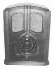
ZENITH MODEL 9-S-232 - Now also known as a "Walton" radio, this ca. 1937 set is the export version employing 9 tubes. It does not have the motorized tuner but does have a selectable operating voltage and a phono input on the rear of the chassis. (Herb Parsons - Peabody, MA)
