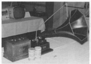
This Edison Gem cylinder phonograph - with original cover, boxed cylinder records and a large crane-mounted horn - was entered in the Old Equipment contest.
