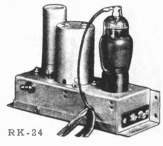
Figure 3. The RCA RK-24 phonograph oscillator. (Photo from "RCA Victor Service Data, Vol. 1," p. 281-B)
