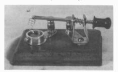
Figure 8. A replica of the Murdock detector.
