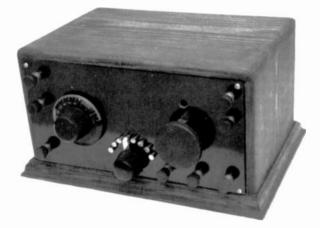
Figure 1. The restored Eaton single circuit set.
