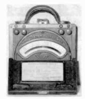
Model 45 - An early System Weston DC voltmeter, last patent date 1898.
