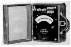
Model 370 - An AC/DC ammeter, standardized date 1916. The instruction sheet is attached to the inside of the cover lid.
