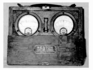
Model 441 - A volt-ammeter combination, date of manufacture unknown, but very old.
