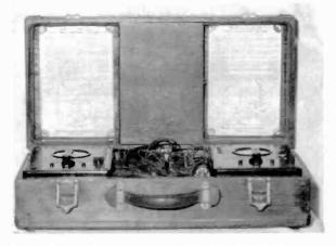
Model 664 - An AC volt capacity meter, standardized date 1930, and Medel 665 - A DC VOM, standardized date 1935. Although sold separately, these models were packaged together in a Type CV case as a test repair kit.
