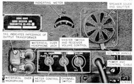
Figure 2. Radio Receiver and Transmitter BC-659, panel view.
