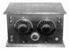
PILOT RADIO – This battery set was probably produced in the early 1920s as a kit. No name appears on the set, but all the components are made by Pilot. It employs a reflex circuit and performs extremely well for a 1-tube set. (Herb Parsons – Peabody, MA)
