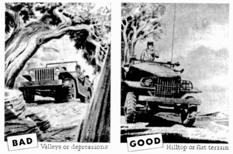
Figure 3. Selecting a proper site for the radio set.
