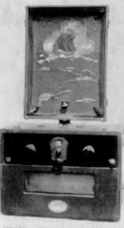
**1927 HYATT –** This 6-tube portable using 6 Type 199 tubes was manufactured by Hyatt Electric and sold for \$120. (Fred Schultz – Ligonier, IN)
