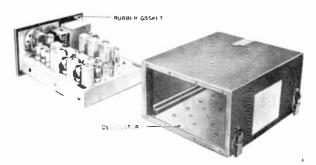
Figure 6. Radio Receiver and Transmitter BC-659, interior view.
