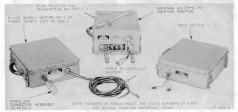
Figure 5. The Radio Set SCR-609 consists of the BC-659 and the plate or power supply unit on the left. The SCR-610 consists of the BC-659 and the battery case on the right.
