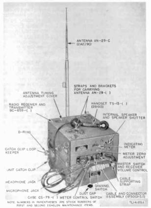
Figure 1. Radio Set SCR-609, assembled for operation.
