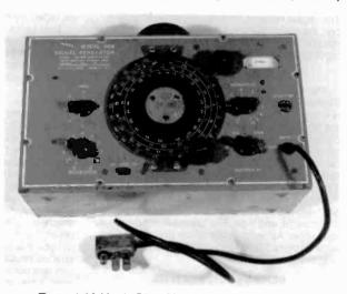
Figure 4. McMurdo Silver Model 906 signal generator.
