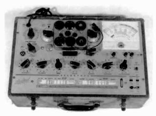
Figure 3. Hickok Model 6000 dynamic mutual conductance tube tester, one of the best for the vintage radio hobbyist.
