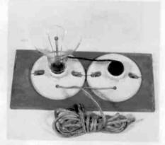
Figure 1. Series light tester, a simple homemade device that will protect your radios and your housel
