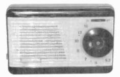
GLOBAL (MODEL NUMBER UNKNOWN) – This Japanese 4-tube superhet uses tube Types 1R5, 1Y4, 1S5 and 354, a 11/2-volt A battery and a 45-volt B battery. The small cabinet is on attractive deep green and cream color. (George Hausske – Wheaton, IL)
