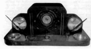
MAKE & MODEL UNKNOWN – This unusual Art Deco style desktop set has AM/SW, a clock, temperature and relative humidity gauges, a pen and pencil set, an inkwell, ashtrays, and a light-up globe dial face. Although the make and year are unknown, the brass plaque indicates the set was an award for the 1936 Employee of the Year at Kelvinator Co. (Rolf Wasseman – Merrick, NY)
