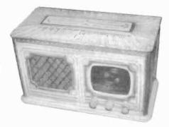
EMERSON MODEL AM-187 – This AM/SW 5tube set is in an antique white Repwood cabinet. The tubes used are Types 6A7, 6D6, 6Q7, 25L6, 2525 and a L49BG ballast. (Joseph Kwoka – Delran, NJ)
