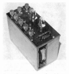
Figure 4. The Weconomy amplifier unit for use with Model 44001.
