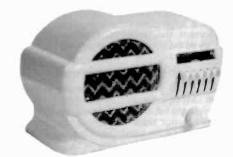
BELMONT MODEL 519 – This 1938 Deco radio features push buttons and has a 5-tube AC/DC chassis. (Alexandria Nelson – Albuquerque, NM)
