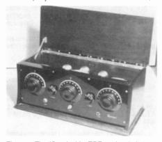
Figure 1. The "Carnival," a TRF 5-tube, 3-dial set, ca. 1924. The New York address on the instruction card later became the address of the Diva Radio Corp.
