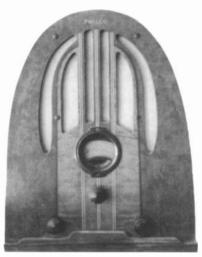
PHILCO MODEL 37-34 - A 5-tube farm set with a vibrator power supply designed to be powered from a 6-volt storage battery, this 1937 cathedral works well. (*Bill Harris - Roanoke, TX*)
