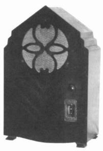
U.S. RADIO & TELEVISION CORP. "SCREEN GRID" MODEL 27 – Schematically similar to the more popular Gloritone model, this 5-tube 1930 model has an inverted chassis. Oil-filled filter capacitors are enclosed in copper cans. (Bob Lackey – Carlsbad, CA)
