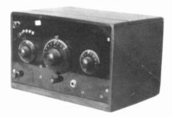
TRI-CITY MANUFACTURING COMPANY MODEL W-4 – This 1923, roughly built 1-tube regenerative set has unique features on the panel. The tap switch shaft is concentric, with the knob controlling the spiderweb regeneration control. Connected below the tuning knob is a vertical bar attached to a much smaller knob. When this small knob is pushed down and turned to the left or right, it acts as a fine tuning vernier control. (Walter V. Worth – Wollaston, MA)
