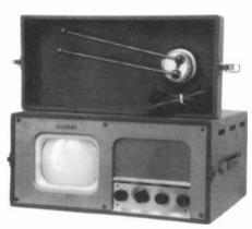
CROSLEY MODEL 9-425 – This 1949 portable television has a leatherette case, two chassis and 20 tubes. The antenna is attached to the front cover lid. (Tony and Lynn DeMara – Mt. Clemens, MI)
