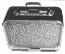
CBS-COLUMBIA MODEL TR-260 — Made of wood with brass trim, this 1959 portable radio has a suitcase design. (Alexandria Nelson — Albuquerque, NM)
