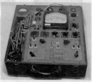
Figure 2. The Hickok 550X Dynamic Mutual Conductance Tester.
