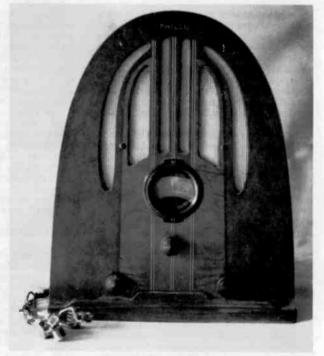
Figure 1. The Philco Model 37-34 farm set uses a vibrator power supply designed to be powered by a 6-volt auto battery. The battery clips can be seen at the lower left of the photo.
