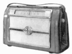
DUCRETET-THOMSON MODEL TR854 – This circa 1962 transistor portable by the well known French company has 3 bands, AM/SW and LW, as is common in Europe. The case is built of molded plywood and covered in fine leatherette. (Walter V. Worth – Wollaston, MA)
