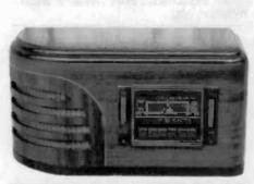
GENERAL ELECTRIC MODEL HJ-624 – The rounded end and distinctive inlaid veneers make this 1939 set very attractive. It uses 7 tubes, one of which is a ballast tube. Although seemingly out of place In larger cabinets, its compact chassis was also used in console Model J-65 and others. (Spencer J. Doggett – Washington, MI)
