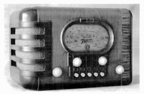
Figure 2. AC-operated sets like this 1939 Zenith Model 5-S-319 displaced the older battery radios. Folks could then enjoy listening to the radio all day without fear of running down a battery.
