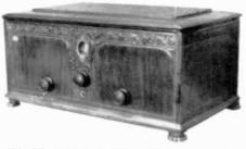
KOLSTER MODEL K20 – This AC set, circa 1925, is In stark contrast to the earlier Kolster battery sets. This set contains no pot metal; it is all cast aluminum. Kolster must have recognized the deficiencies of the 6D-6K models and corrected them. (Walter V. Worth – Wollaston, MA)
