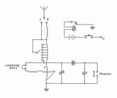
Figure 8. Schematic for the GECoPHONE No. 2.
