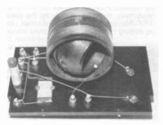
Figure 4. Interior view of the GECoPHONE No. 1 Crystal Set.
