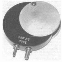
Figure 3. GECOPHONE loading coil with adjustable aluminum vanes. Three different ranges were available; this one was designed for 1200-1850 meters for reception of the Paris Radiola station.
