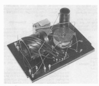
Figure 7. Under-panel wiring of GECoPHONE No. 2.
