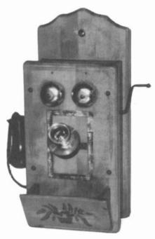
MASTERS ART MODEL 220 - This early Japanese tube-type wall phone novelty radio uses the bells for on/off and tuning, similar to the transistor radio units manufactured later. (Gary Amold - Marion, NC)
