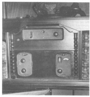
Figure 11. The Radiola 64 panel in the Victor 9-54. The bezels are unique to the 3 Victor models.
