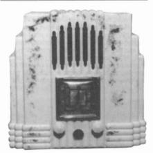
AUSTRALIAN RADIO MODEL UNKNOWN – This 1937 set resembles the Air King Skyscraper. The ¼" thick white Bakelite cabinet with orange and black marbleized design measures 11" x 10½" x 6". The 5-tube chassis uses Type 80, 42, 6B7, 6D6, and 6A7 tubes. (Tom Romano – Millbury, MA)
