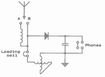
Figure 5. Schematic for the GECoPHONE No. 1.
