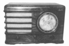
INGELEN RADIO – This pre-World War II German table model features a map of Europe. The ring surrounding the map has the names of many European cities. The two outer rings bordering the bezel appear to carry station call letters and frequencies. A unique tuning mechanism tracks and locates the desired station and frequency. (B. Pickell and G. Levine – Greenlawn, NY)
