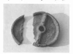
Examples of cracked castings. Left: Crosley tuning dial assemblies for early AC sets. Right: Atwater Kent dial pulley.
