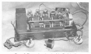
Figure 8. The receiver chassis of the Radiola 67.
