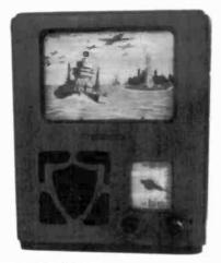
RADIO VISICN MODEL 414 – This 5-tube, AM, AC/DC set, ca. 1940, has a chassis manufactured by M.R. & T. Corp., Chicago. The action unit makes the picture come alive when the radio is on. (Michael Hilton – Tucson, AZ)
