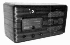
GENERAL ELECTRIC MODEL F-74 – This set has been restored but does not have the original grille cloth. It features a tuning eye and broadcast and shortwave bands. Because the speaker is on the right and the knobs on the left, it is sometimes referred to as a left-handed radio. (Arthur Kreitner – Belleville, IL)
