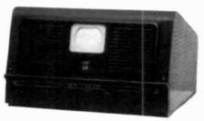
PILOT MODEL TV-37 – This 1949 TV used 17 tubes with a 3-inch picture tube. At \$99.50, it was the first TV priced under \$100. (Tony DeMara – Mt. Clemens, Mt)
