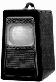
SENTINEL MODEL 400 - This 1948 leatherette portable TV uses 2 chassis with 20 tubes and a 7" picture tube. (Tony and Lynn DeMara - Mt. Clemens, MI)
