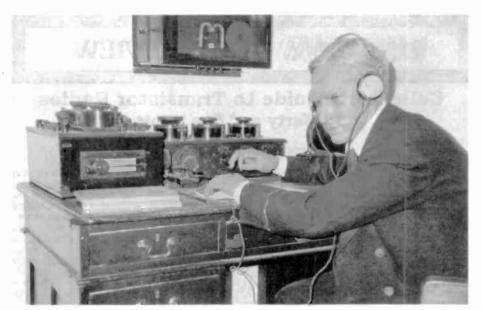
Figure 2. Diorama of an early 1900s Marconi shipboard receiver/transmitter. You may notice that the operator is wearing 1920s Federal headphones rather than a more appropriate pair from the teens.
