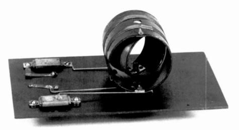
Figure 3. An interior view of the radio showing the variometer and capacitors mounted on the rear of the front panel.
