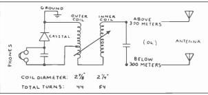
Figure 4. Schematic for the Radiola I.
