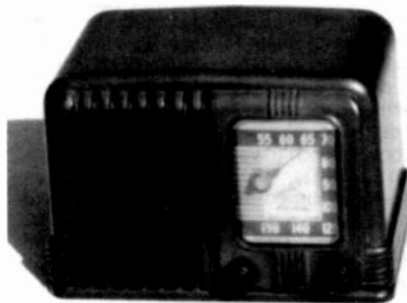
The RCA 45X11 5-tube superhet in a mahogany brown, plastic Art Deco cabinet.
