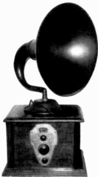
MOHAWK CHEROKEE – Made in Chicago, ca. 1925, this 1-dial, 6-tube battery set uses (5) Type 01-A tubes and (1) 200-A tube on a black Bakelite chassis. This radio uses a Bristol Baby Audiophone speaker and is in nice original finish. (John and Joan Balliett – Muncy, PA)
