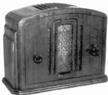
PHILCO MODEL 57 – A real signal grabber, this old timer, ca. 1932, has 4 tubes. It receives the old police band, and the band switch is located at the rear of the chassis, next to the trimmers. The tube complement is (1) Type 80, (1) 42, and (2) 77s. (Joseph C. Burke – Weehawken, NJ)
