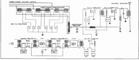
Circuit diagram of the single sideband carrier eliminated transmitter, from Mary T. Loomis, "Radio Theory and Operating," p. 430.
