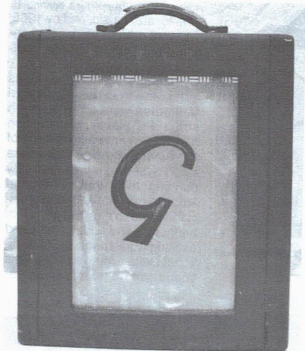
Figure 3. The Gibson BR1, named for the designer Barnes Reincke, has a 12-inch field-coil speaker.
