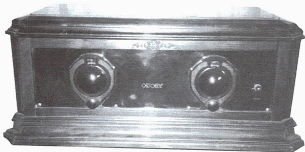
NUNN-LANDON – Made in Milwaukee, this set has 5 tubes — (3) Type 201As and (2) Type 112s. It also has a Bakelite chassis with tube sockets that have vibration reducing mountings. (Mike Nall – Grayslake, IL)
