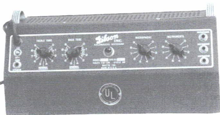
Figure 2. The Gibson EH185 amp, ca. 1937, has a 12-inch field coil speaker and a removable chassis.
