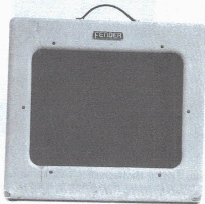
Figure 5. The Fender Pro amp with tweed covering has a cabinet called the "TV front."
