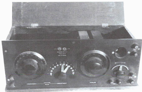
GREBE CR-5 – This set, manufactured in Richmond Hill, N.Y., is an early version of the CR-5, with the tube exposed and an open rheostat. ( Will Jensby – Santa Clara, CA )
