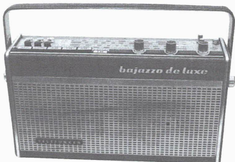
TELEFUNKEN BAJAZZO DELUXE – This teakwood case German portable has AM/FM, two SW bands, and multivoltage or 6 D cells. It features 3 FM preset push buttons, each with its own tuner. (Randy King – Lincoln, NE)
