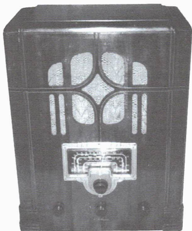
RCA VICTOR TOMBSTONE MODEL 8BT – This 8-tube battery set, manufactured in 1938, features three bands and is in completely original condition. ( David Wiggert – Onalaska, WI )
