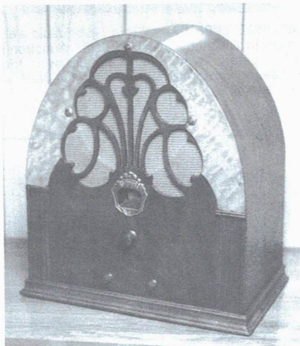
Figure 2. The Philco Model 20 Deluxe cathedral with a curly maple arch and columns.
