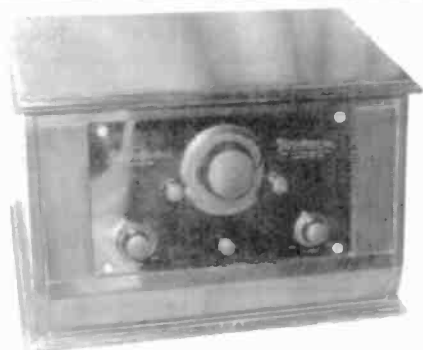
DISTANTONE "FIVER" - This 1926 battery set, made in Lynnbrook, N.Y., has a slope front made from a high glass, deep maroon-colored Bakelite panel. It is a single-control radio with all tuning capacitors on one shaft directly driven by the large center knob. The radio is in excellent condition and is on display at our museum. (Vintage Radio & Communications Museum - New Britain, CT)
