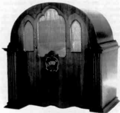
CROSLY MODEL 124 “PLAYBOY” – Described in Rider's as a compact 10-tube superhet, this gem was only in need of a good cleaning and new filter caps when I found it in New Bedford, Mass. All tags are in place, and it plays beautifully. The tube complement is (1) Type 80, (2) 27s, (2) 35s, (2) 24s, and (2) 47 push-pull output tubes. ( Joseph C. Burke – Weehawken, NJ )
