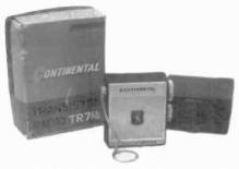
CONTINENTAL MINI-TRANSISTOR RADIO – This 7-transistor model uses a penlight battery and measures 2 ½" by 2 ½" by 1" deep. It has a brushed aluminum face, a key chain, and a vinyl carrying case. (Randy King – Lincoln, NE)
