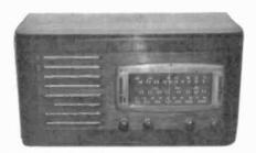
FARNSWORTH MODEL BT1010 — This imposing 10-tube AC set from the late 1940s has two push-pull Type 6V6 output tubes and an 8-inch dynamic speaker. Note the unusual slider-type bass and treble vertical tune controls on either side of the dial escutcheon. (Gregory E. Jones — Westerly, RI)
