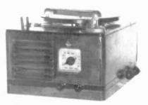
EMERSON "LITTLE MIRACLE" - This Emerson Radio-Phono, ca. 1938, uses the "Little Miracle" chassis, a high quality astatic tone arm, and a center drive gear-driven turntable. It was a nice little package in its day for \$19.95. (Barry Cheslock - Arlington, VA)
