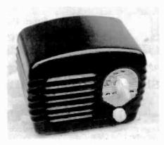
Figure 5. The 4-tube Arvin Model 442.
