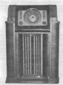
CROSLEY MODEL 03CB — This large 10-tube floor model, circa 1940, with a waterfall front and a 12-inch speaker, has six push-button station settings and six push-button tone control positions, as well as 2 shortwave bands and a broadcast band. (Randy King — Lincoln, MF)
