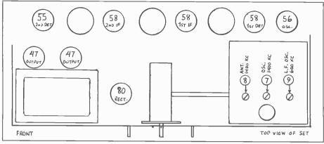
Figure 4. Sketch of top view of the Silver-Marshall chassis showing location of the trimmers.
