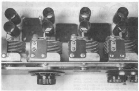
Figure 3. Top view of the Atwater Kent Model 33 chassis. Note the metal loops in back of the knobs, used for ganging the 4 tuning condensers.
