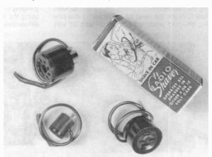
The Radio Shaver Model 200. Clockwise from top right: the original container, the female 110-volt socket for the dashboard, the 7-pin miniature socket, and the octal tube socket.
