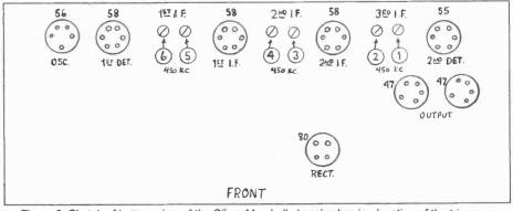
Figure 3. Sketch of bottom view of the Silver-Marshall chassis showing location of the trimmers.
