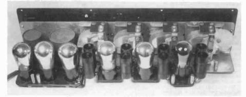
Figure 2. Rear view of the Atwater Kent Model 33 chassis. Note the trimmer condenser at the far right.
