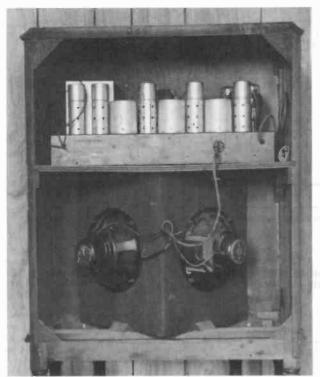
Figure 2. Rear view of the Silver-Marshall Model Y. Notice how the twin Jensen speakers are installed.
