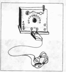
Figure 1. A drawing of the simple crystal receiver offered to the author in 1922. It consisted of a tapped tuner with a catwhisker type of crystal detector, a Murdock fixed condenser, a pair of 2.000-ohm Murdock phones, 200 feet of No. 14 copper antenna wire, two 4-inch insulators, and a ground strap. It had a range of 200 to 3,000 meters. However, the \$16 price tag was beyond the author's means at the time.
