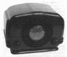
CORONADO MODEL C5D14 - This miniature Bakelite radio (8" wide x 5 1/2" high) was manufactured about 1941 or 1942 by the Gamble Skogmo Company. The schematic for this 5-tube AC-DC set is in Riders, Volume 13-3, 4. (John Schehrer - Joplin, MO)
