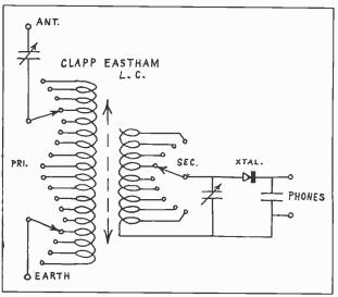
Figure 4. Schematic diagram of the Clapp-Eastham receiver.
