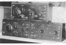
These Crosley sets are the 3-tube Model 52 receiver, the 1-tube Type V receiver and the 2-tube Type IV audio amplifier.
