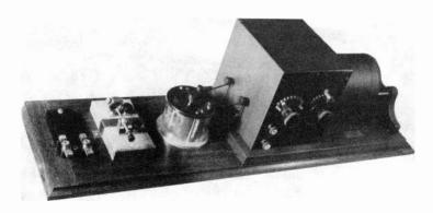
Figure 3. The Clapp-Eastham loose coupler set.
