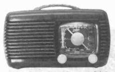
ZENITH MODEL 6-D-510 - This brown Bakelite set was my first old radio, circa 1940. It uses the Zenith box-loop antenna with RF amplification via a 12J7-type tube. (Colin Stump - Lancaster, OH)
