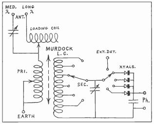
Figure 2. Schematic diagram of the Murdock receiver.
