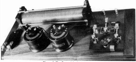
Figure 5. The Bunnell 3-slide tuner set.
