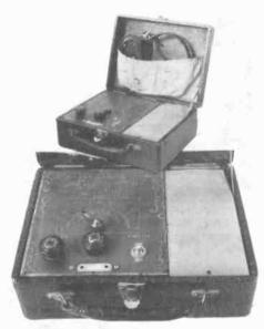
BROTHER SUPER REGENERATIVE SET - This Japanese portable was made in the mid-1930s. It used two space-charged Type UY-111B tetrodes for super regenerative detector and audio amplifier. (Noriyoshi Tezuka - Tokyo, Japan)
