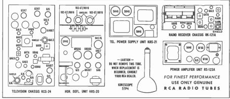
Figure 3. Chassis diagram of the RCA Model 684PTK projection TV showing the tube layout.
