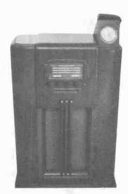
GENERAL ELECTRIC MODEL G97 - Note the timer clock mounted in the upper right hand corner of the cabinet. This model has the AM band plus two shortwave bands. (Bill Graham -Aurora, NE)
