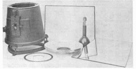
Figure 5. The Model 648PTK optical projection system components.
