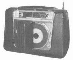
**METZ PORTABLE RADIO-PHONO** - This German-built radio from the late 1950s has three bands (SW, MW, LW) and a built-in 45 rpm turntable behind an opening front panel. The set works on battery or 110-240 volts and includes the original 2-prong German Mains plug. An album located inside the removable back panel holds ten 7-inch records. (Steve Kissinger - Thousand Oaks, CA)
