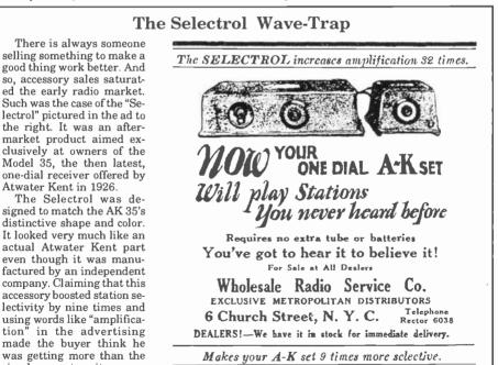
A wave-trap is a device consisting of a coil and variable condenser in series with the antenna circuit to get rid of interfering signals from strong local stations.
