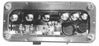
Figure 3. Bottom view of the AK Model 35 showing the chassis components and tubes.
