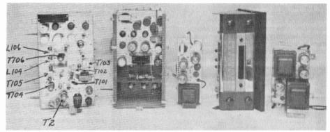
Figure 2. The five electronic units of the Model 648PTK. From left to right: the TV chassis, the horizontal deflection chassis, the TV power supply, the radio chassis, the audio and radio power supply.
