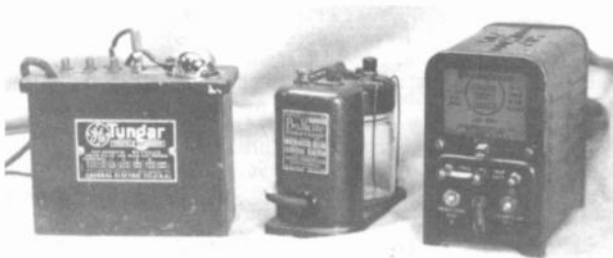
Figure 3. Right: Westinghouse Trickle Charger, 6v at \frac{3}{4} amp. Center: Balkite Trickle Charger, 6v at \frac{1}{2} amp. Left: GE Tungar Trickle Charger, 6v at \frac{1}{2} amp.
