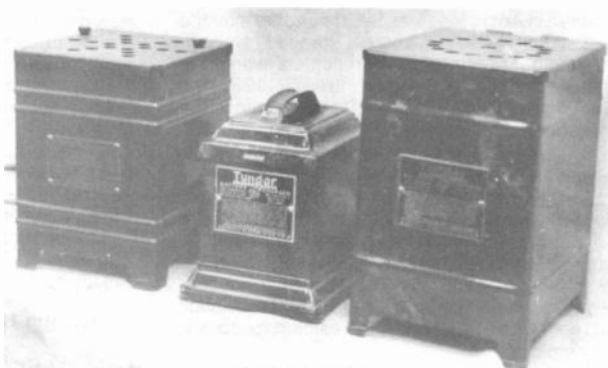
Figure 1. Right: GE tungar battery charger, 3 cells at 5 amperes or 6 cells at 3 amperes. Center: GE Tungar charger, 3 cells at 5 amperes, 6 cells at 3 amperes or 40 cells at ¼ ampere. Left: Westinghouse Rectigon charger, 2 to 96 volts at 2 amperes to ¼ ampere.
