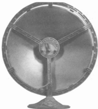
HERALD CONE SPEAKER - This speaker has a lever in the center to adjust the tone. The small metal body is finished in bronze and lamp black. The driver is hidden behind the tone control plate. (Fred Geer - Jacksonville, FL)
