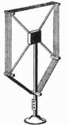
Figure 6. An illustration from "Radio News" of the loop aerial construction recommended for use with the kit.
