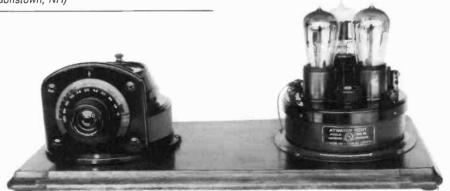
**ATWATER KENT 3945** - This early breadboard receiver uses a 3-tube TA unit and a Type 11 tuner. Space is left between them for an AK variometer to make this set regenerative. (Kurt Nauck -Houston, TX)
