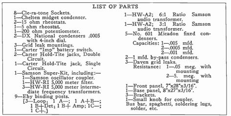
Figure 1. The list of parts and materials required to assemble the Samson Super-kit.
