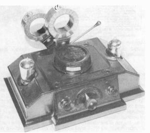
Figure 6. Brownie 2-valve receiver with Mullard dull-emitter type valves.
