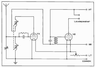
Figure 7. Circuit diagram of Brownie 2-valve receiver.
