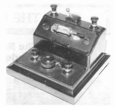
Figure 8. Brownie No. 3 crystal set. A wave-change switch replaces the plug-in coil of the No. 2.
