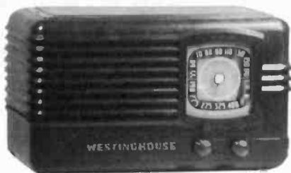
WESTINGHOUSE - This set, model number unknown, is a typical ultracompact radio built in 1940. The slim cabinet is an illusion as the cardboard back sticks out 1.75". (Fred Geer - Jacksonville, FL)
