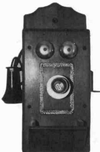
WALL TELEPHONE RADIO - This novelty receiver of ingenious design employs the bells for on-off/volume and tuning. It has a wooden cabinet and a rectangular speaker grille. A great conversation piece! (Peter Oppenheim - New York, NY)
