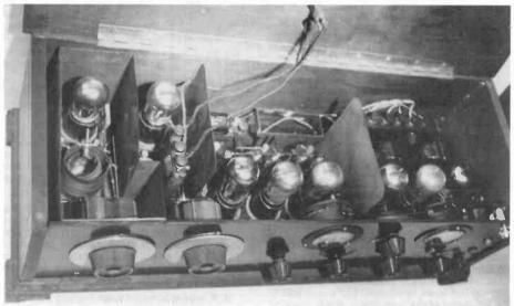
Figure 3. Internal view of the Popular Mechanics' Superheterodyne Eight showing the copper shielding throughout, as well as the Remler components.
