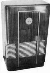
SPARTON MODEL 1486 - Note the stunning cabinet of this 1936 model made with ribbon mahogany and trimmed with brass strips. The speaker grille is accented with horizontal rows of brass tubing. The radio dial and knobs are behind two doors. A fourteen-tube radio on two chassis, it has one twelve-inch speaker and two three-inch tweeters. (Doug Heimstead - Fridley, MN)
