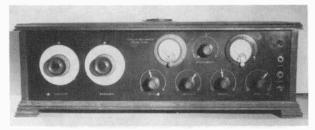
Figure 1. The completed Popular Mechanics' Superheterodyne Eight receiver made from the factory kit.
