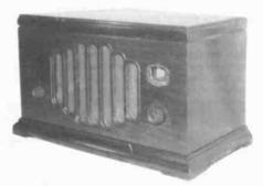
FADA MODEL 55 - This set was made by the Fada Radio and Electric Co. shortly after D'Andrea went bankrupt, and the company name had changed. The set weighs a hefty 23 pounds with a large AC transformer and a nine-inch dynamic speaker. Inside are Fada tubes, installed when new. It needed no repairs to play. (Walter Worth - Wollaston, MA)
