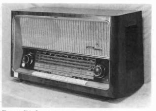
Figure 4. This Grundig Stereo 4192, a 10-tube 5-band set with four speakers, covers the 11 to 125 meter shortwave bandwidth. It has a Multi-Sonic sound system and is 25-inches wide.
