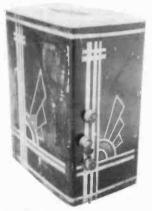
RCA MODEL R-28-BW - This 1932 style radio is 20 1/2" high by 8" by 12". The sides are covered with a one-piece tin plate whch is fitted flush under the wood top. A Deco design is stencilled on all sides in black. The top, which holds the speaker, is painted silver. The back cover, missing on this one, was apparently also tin plate. It has standard RCA wood knobs and a small dial opening. (Steve Lange -Milwaukee, WI)
