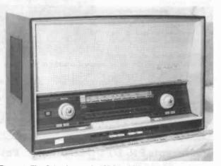
Figure 1. The Saba Automatic 125 is a 28-inch wide, 13-tube radio with five speakers and four bands. It has automatic motor tuning with a signal-seeking feature.
