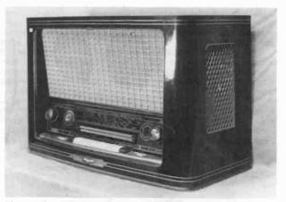
Figure 5. The Saba Meersburg 7 is a 10-tube, 4-speaker receiver with four bands and automatic motorized tuning. It is 25-inches wide and is typical of the quality-built sets of 1962.
