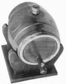
RADIO DEVELOPMENT AND RESEARCH CO. MAGIC TONE - This keg radio is in a ceramic, rather than wood, container. The spicket is actually the on/off switch and volume control, while the plug on top is the dial. (David McKenzie - Eustis, FL)
