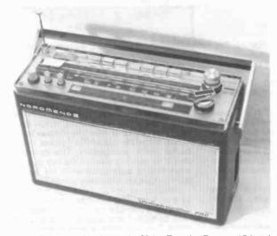
Figure 3. This 1964 Nordemende Globe Traveler Pro – a 15-band (11 to 80 meters) portable with 29 circuits and a 6-inch by 9-inch speaker — weighs 11 pounds and includes every important feature and the finest multiband engineering.
