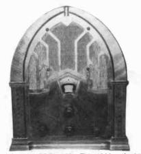
**CROSLEY MODEL 168 -** This 1933 cathedral radio is a seven-tube dual band superheterodyne. The intermediate frequency is 181.5 Kc. *(Lyle Scheid - Iroquois, SD)*
