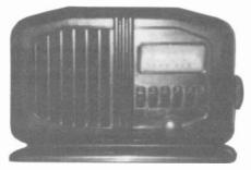
TRUETONE MODEL D1011 - This brown Bakelite table set was manufactured by the Belmont Radio Corporation. Note the simple but graceful lines of the cabinet, accentuated by the six push buttons between the rectangular dial and the on/off switch-volume control. The tuning knob is located on the right-hand side of the cabinet. (Dave & Terry Masterson -Cheshire, CT)
