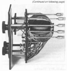
Figure 3. Type RA. Inside view showing variable capacitor and variable inductance on a common shaft. (Photo courtesy of The Vestal Press)
