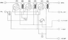
Figure 15. Schematic for the AR RF amplifier.
