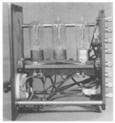
Figure 8. Chassis view of Type DR showing use of WR-21 A and WR-21 D Aeriotron tubes. (Photo courtesy of Lauren Peckham)
