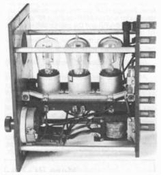
Figure 4. Type DA. Note center deck for tube mounting. Audio transformers are secured to rear panel. (Photo courtesy of The Vestal Press)
