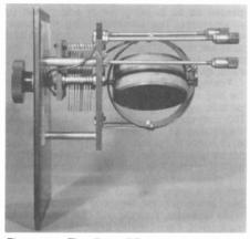
Figure 11. The Type RT. Inside view shows same tuning system as used in the RA except that the fickler coil winding is omitted. (Photo courtesy of Lauren Peckham)
