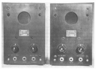
Figure 7. The almost identical Westinghouse resistance-coupled DR on the left and the transformer-coupled DA on the right. You must read the nameplate designation to distinguish one from the other.
