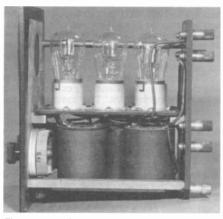
Figure 13. A view of the Type AR chassis. Note the three, large, Micarta-covered radio frequency coils. (Photo courtesy of Lauren Peckham)
