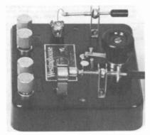
The later version of the DB Crystal Detector. (Photo courtesy of The Vestal Press)
