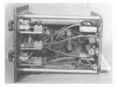
Figure 9. Bottom view of Type DR. Note the glass-enclosed resistors tucked under the subpanel. Large carbon-rod resistors are mounted on the rear panel along with the two coupling capacitors. (Photo courtesy of Lauren Peckham)
