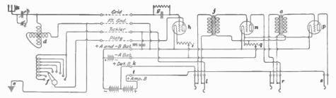
Figure 5. The schematic for the Westinghouse RA and DA, and the Type RC receiver, as shown in the "I.C.S. Radio Operator's Handbook" of April 1923.
