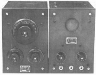
Figure 2. Westinghouse Type RA regenerative tuner on the left and Type DA detector-amplifier on the right. (Photo courtesy of The Vestal Press)
