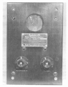
Figure 12. Front panel view of the Westinghouse Type AR radio frequency amplifier. (Photo courtesy of Lauren Peckham)
