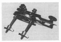
PATRICK & CARTER LANDLINE KEY - This massive brass leg key was made during the 1870s for work, not for show. These keys were attached through the tabletops so that the wires connecting to the rest of the telegraph station would be out of the way of the operator whose desk was usually very deeply buried in traffic. (*Photo courtesy of Bill Holly, K1BH*)
