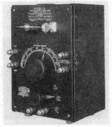
Figure 2. The 1922 RCA Radiola Concert Receiver crystal set Model AR-1375.
