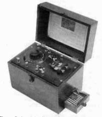
Figure 2. Another view of the Edison Bell Type B Crystal Set, showing battery compartment.
