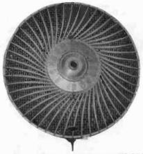
TOSHIBA WALL-MOUNTED TRANSISTOR RADIO - This highly unusual radio was made especially for wall mounting. This seventransistor set is twelve inches in diameter and gold in color. Note the pull-chain switch on the bottom and the double-printed dial which enables the operator to read the dial from a reclining or standing position. (Victor Marett -Miami, FL)
