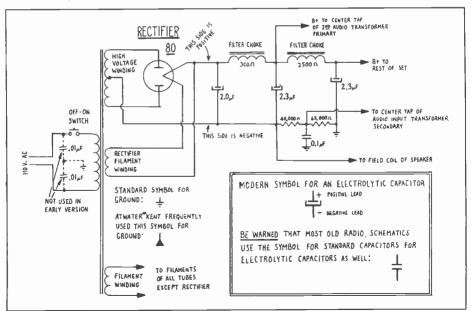
Figure 1. Power supply circuit of the Atwater Kent. Model 55 receiver.
