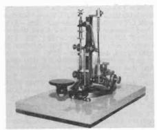
THE VAILOGRAPH - This is an attachment which neatly slipped onto the myriad of steel lever keys found everywhere in the telegraph community. Dashes were made in the normal manner, but with this device attached, repeating dots could be made by lifting up on the knob of the key. It was an inexpensive way of converting a key into a bug. I have seen only one other of these, in the Ford Museum. (*Photo courtesy of Bill Suter*)
