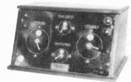
MICHIGAN M10 - The Michigan Radio Corp. of Grand Rapids, Michigan, made this one-tube regenerative set in 1923. It is of very light construction with a formed aluminum panel and has room inside for A and B batteries. (Walter Worth - Wollaston, MA)
