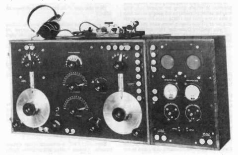
Figure 4. Atlantic Radio Company also sold this Wireless Specialty Co. Type IP-500 (SE-143) and matching two-tube Type B Amplifier.
