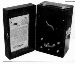
**RADIOLA I PORTABLE - This is the** Model ER-753A crystal receiver by RCA. The panel is stamped but not filled with a whitener, which makes it difficult to read. The rear compartment is for storage of Murdock headphones, which were recommended by RCA. The thin leather carrying strap is usually missing, and often the detector unit has been replaced by a more sensitive type. (Dave Crocker -Duxbury, MA)
