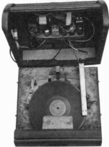
Figure 2. Note the wood screws on the sides of the frame which lock the radio cabinet in place.
