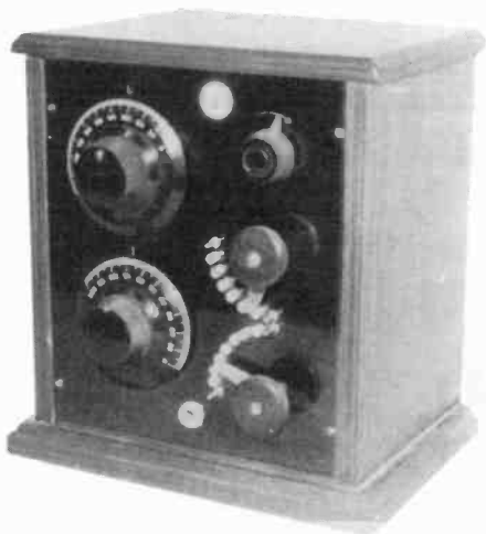
HOME BREW RECEIVER - I made this one-tube regenerative radio to look like the Clapp-Eastham R4 receiver. All old parts were used, and the cabinet is of oak plywood with oak veneer banding in the edges. (Walter Worth - Wollaston, MA)
