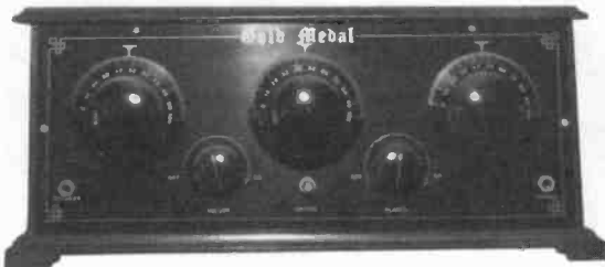
GOLD MEDAL - This three-dialer was made in 1925, and was sold as the Gold Medal Deluxe. It used five tubes and its price was $90. (Mike Adams - Scotts Valley, CA)
