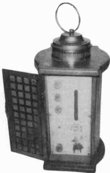
GUILD TOWN CRIER LANTERN - This seven-tube radio has a unique colonial lantern design. The solid woods used in the cabinet are complemented by four wooden knobs. The metal lattice-work door contains a simulated amber glass front. The tube complement has a 35EH5, 12AV6, 12BE6, 12BA6 (2) and a 17EW8. This mint condition set has excellent sound. (Ken Armstrong - Storm Lake, IA)
