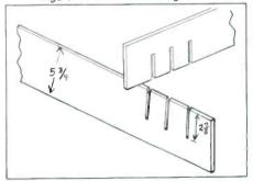
Figure 2. Alternating sections cut and ready for assembly.
