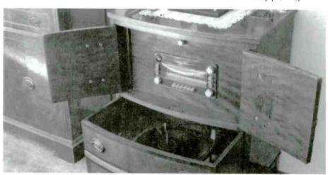
Figure 8. The Tempotone Model 1036 opened for radio/phono operation.
