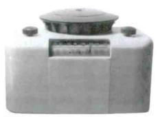
UNIQUE SPEAKER RADIO - This is the International Kadette "Topper," ca. 1940. It may have been the last plastic radio manufactured by this company. It featured a speaker on top with a deflecting dome to diffuse the sound in all directions. The cabinet is ivory with a brown top and brown knobs. The chassis is inverted. (David Mednick - Fort Lee, NJ)
