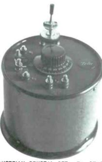
AUSTRIAN CRYSTAL SET - The OTAG Type LOLO was produced in Vienna in 1926. Its original plug-in detector was called "LUX." (Erwin Macho - Vienna, Austria)
