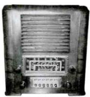
CROSLEY TABLE MODEL - The broadcast band and shortwave receiver has an all-wood cabinet. It features push buttons for station tuning. The model number is unknown. (David Masterson - Mexiden, CT)
