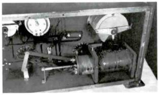
Figure 2. Rear view of the audion tube receiver showing the components used in the construction.
