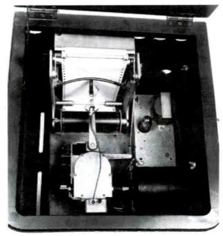
Figure 3. The interior of the Crosley Reado facsimile printer showing the stylus mechanism. The tube, visible to the right, is a Type 0Z4.
