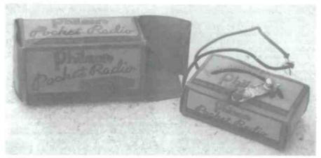
PHILMORE POCKET RADIO - This compact set Is equipped with a fixed detector and slidewire. The phone plugs are on the side. The wires are connected to the antenna leads. The Pocket Radio fits neatly into its hard paper container. The color is green, black and gold. (A. R. Nolf - Ontario, Canada)
