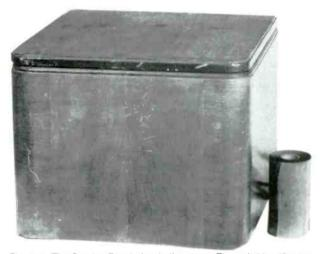
Figure 1. The Crosley Reado facsimile printer. The only identification is a small "Crosley Reado" decal on the front.
