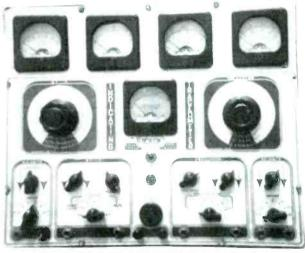
Figure 1. The Hickock Model 155 Radio Traceometer.
