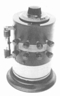
Figure 3. The rear of the receiver showing the paper label stating its manufacture by the Clapp-Eastham Company. The Myers detector-amplifier tube is shown to the left, held in place by the two socket clips. Also shown are the binding posts for the antenna and ground, for the A and B batteries, and for the headphones.
