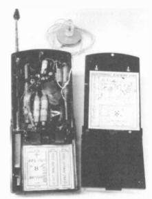
Figure 2. Privat-ear Pocket Radio with the rear cover removed.
