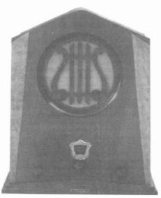
GILFILLAN RADIO - This early 30's cathedral was manufactured by Gilfillan. It looks like a Jackson-Bell Model 62, but has a small metal tag on the lower front that reads "Tiffany Tone." It has a six-tube TRF circuit. (John S. Neuman-San Carlos, CA)
