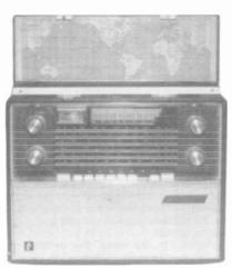
AM/FM TRANSISTOR RADIO - This six-band 16-transistor radic was made in Japan for the J. C. Penney Co. This Model 1903 is a very powerful set. Note the world map, which though useful then to log stations, is now likely obsolete! (Norm Landis - Kirkwood, MO 63122)
