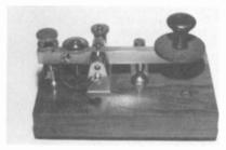
FRENCH SPARK ERA KEY - This spark era key was made by the DuCretet & Rogers Co. While it is not the heavy, massive construction of the "Rock Crushers" from Marconi, it did the job fairly well. A slightly larger version of this key used oil break contacts. Photo courtesy of Neal McEwen, K5RW
