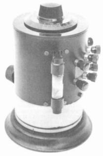
Figure 4. The Myers tube, in position on the receiver, has one red and one black Bakelite end cap. The top is enclosed with a black Bakelite cap on which is a dial for tuning.
