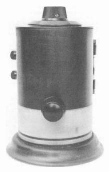
Figure 2. The front view of the Clapp-Eastham regenerative receiver, quite possibly the Billow model. Its construction is of a black Bakelite cylinder mounted on a turned wooden base. Wound around this cylinder is white cotton-covered wire that terminates just below the regeneration control knob.
