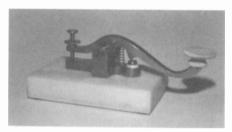
THOMAS HALL CAMELBACK - This simple but effective early instrument uses ivory for the knob and insulator. It dates from about 1848, and is a good example of the curved camelback keys of that period. Although originally found on a wooden base, this example is now mounted on marble. Photo courtesy of Bill Holly, K1BH
