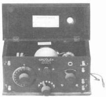
EARLY CROSLEY - Offered in 1923, this onetube Model V appeared in this early style box with overhanging lid. The hole in the lid was drilled at the factory to accommodate the added height of a tipped tube (such as a WD-11) used with an adapter. (Dave Crocker -Duxbury, MA)
