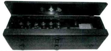
RADIOLA 18 - The Radio Corporation of America (RCA) manufactured this AC receiver in 1927. It is a seven-tube TRF that sold for \$115. (Norm Landis - Kirkwood, MO)
