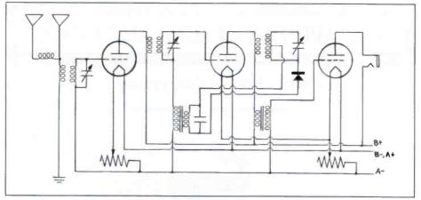
Figure 3. Circuit diagram of the Edison Model R-3. (Drawn by Norman Braithwaite)
