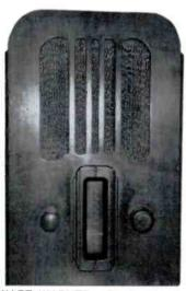
STEWART WARNER - This tombstone is a Model R-3043-A with the following tube complement: 6A8G, 6K7G, 6K6G, 5Y4G and 6Q7G, all of which are Arcturus blues. The unusual feature about this set Is that the chassis is mounted vertically, and the dial is designed so that the set can be operated upright or on its sidel It measures only 12 inches high. (Donald P. Amshay - Durham, NC)
