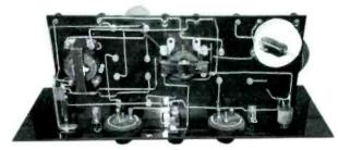
Figure 2. The Edison Model R-3 chassis viewed from below; the basketweave coil is on the right and the crystal detector is at the bottom middle.
