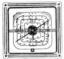
Figure 2. Dial face of the General Electric Model M-81 All-wave receiver.
