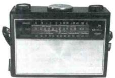
MULTI-BAND PORTABLE - The Wards Airline Model GTM-1233A was a three-band (BC, marine and SW) portable of the 1950s. The leather case slips off straight up to expose the chassis. It is an excellent SW performer, even tocay. (Bob Moore - Lakewood, CO)
