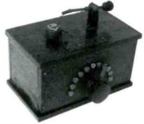
CRYSTAL SET – This is the Type No. 1-B manufactured by the Radiofone Corporation of Detroit, Michigan. It is of ultra simple design and construction, consisting of a nailed wooden box. Its price was a mere \$3.10. (Erwin Macho – Vienna, Austria)
