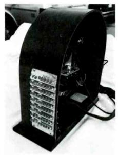
Figure 8. The Scott Automatic Program Selector Clock showing the storage rack for the programming pins.
