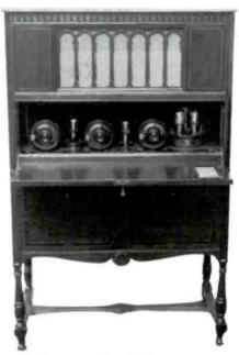
BREADBOARD CONSOLE — This is the Atwater Kent Model 1100 that was sold in a Pooley cabinet. It has a rectangular wooden horn speaker built into the top and a battery compartment below. (George Found — Kitchener, Ontario, Canada)
