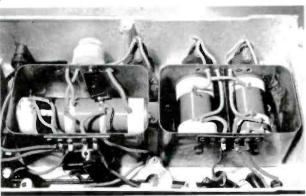
Figure 4. RF coils of Victoreen Type A with box covers removed.
