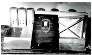
Figure 2. Front of Victoreen Type A chassis showing heavy aluminum casting.
