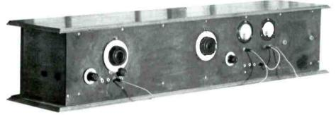
Figure 1. Ten-tube Superheterodyne. Builder and designer unknown. Controls: RF gain; ant. tuning; osc. tuning; IF gain; audio outputs. Lower eight banana plus jacks are for metering each filament voltage; last one reads three audios together. Use a patch cord to the jack under left meter. Right meter is for high voltages. Panel is 47 1/2" by 9".
