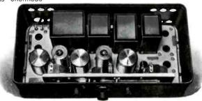
Figure 2. Interior view of the Atwater Kent Model 55 receiver showing the quality of workmanship. (Illustration from the 1929 Atwater Kent advertising booklet).
