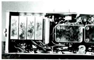
Figure 5. Victoreen Type A chassis showing IF coil boxes (left side).
