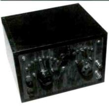
LABELLE MODEL 21 - This dual-tapped crystal set was produced in 1923 by the Labelle Radio Co. of Attleboro, Mass. The panel is orange and black swirr to match the two tap switch knobs. The small center knob rotates the catwhisker on the crystal inside the box. (William Key - Halifax, MA)
