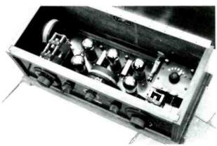
Figure 2. Interior view of the Oriole Model 7B showing the 5-tube layout and the unique antenna coil tap switch to the right.
