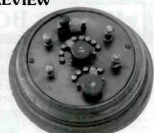
CRYSTAL SET - This home made crystal set is signed "C. Sholtes" on the bakelite panel above the detector. The detector is a combination type. (Frank R. White - Olathe, KS)
