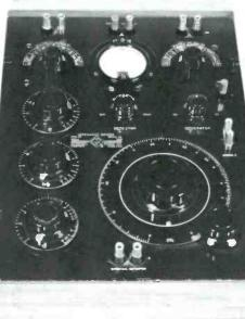
Figure 1. General Radio 650-A Impedance Bridge
