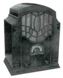
CLARION TOMBSTONE - The Transformer Corp. of America manufactured this 8-tube superhet receiver. It is the Model 80 and sold for \$67.50 in 1931. It had variable-mu and pentode tubes. (William Key - Halifax, MA)
