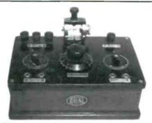
GERMAN CRYSTAL SET - This receiver, manufactured by Lorenz of Berlin, is a Model EDA 24 and was produced in 1924. It is a very rare set in a wood case with the famous Friho crystal detector. It uses variometer tuning. (Erwin Macho - Vienna, Austria)
