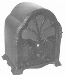
FADA CATHEDRAL - This Model 43 receiver was my 1000th radio! It has seven tubes, a TRF circuit with push/pull output. The front is of Repwood-type of material. (Ron Boucher - Goffstown, NH)
