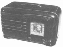
LONE RANGER RADIO - Pilot Radio Co. manufactured this Model B1151 in 1939. The cabinet is of brown bakelite with a handle on top. Pictured on the dial is an illustration of the Lone Ranger riding Silver. It is a superhet circuit using 5 tubes: 1- 65K7, 1- 6SQ7, 1-25L6G and 1- 65A7. (Jane Walackas - Whitman, MA)
