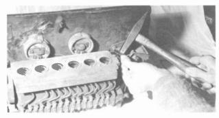
Figure 2. A single-edged razor and hammer is used to cut the seals.
