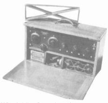
MODEL VIII PORTABLE - Crosley offered their Model VIII in two versions: the standard table cabinet style and this oak portable. It sold for \$96 which included 3 tubes, phones, batteries and antenna wire wound around a wooden frame. (Dave Crocker - Lyndonville, VT)
