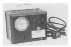
STERLING VACUUM TUBE REJUVENATOR - This has a lever switch for "flash" and "age". Note the early screw plug for an AC transformer. (Walter V. Worth - Wollaston, MA)
