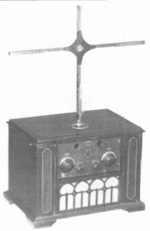
**DEFOREST D12** - This rather large 1924 ser used an internally-mounted catwhisker and crystal for detection along with a four-tube cir cuit for power. Later versions substituted a detector tube instead of the crystal for ease of operation. (*Dave Crocker - Lyndonville*, *VT*)
