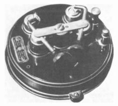
Figure 7. A factory-made Atwater Kent double crystal detector unit from the Editor's collection.
