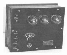
Figure 2. 7A amplifier, panel view.
