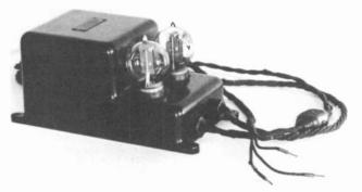
Figure 4. 2A power supply for the 7A amp. (Note: the 2A uses two type 217A rectifer tubes; the critical eye will notice that the rear tube in this photo is a type 216A inserted for appearance since a type 217A was not available.)
